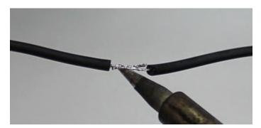
Figure 9: Soldering two wires.
