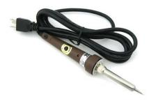
Figure 2: Soldering Iron
